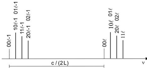
Fig. 10.3 Frequency spectrum of modes of a long resonator
